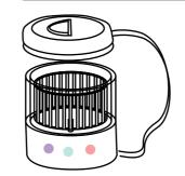
The interior of Munchkins steriliser is 63.6 mm x 63.5 mm so ours must be at least this size.
