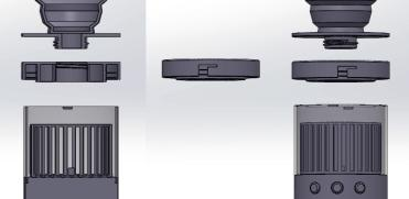
The cross section view tool was used to ensure **geometries** were realistic and successful. A wall thickness of 2 mm was chosen as this is a common size and worked well in the design. There were some problems with interferences of the clear middle with the other parts due to the exact diameter dimensions being used when a small gap would need to be present in the physical product.
