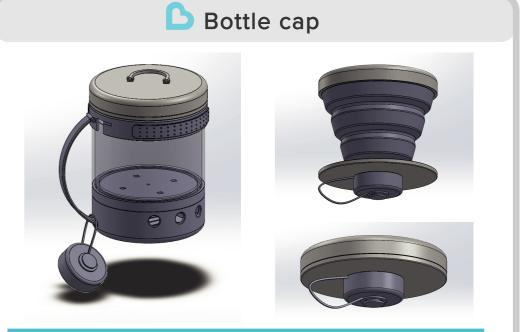
After modelling the cap as drawn in the original concept (attached to top handle), we found that the **attachment** would have to be long to reach the screw top, this would get in the way of the **main product function**. Therefore, the cap was made to be its **own component** that could **attach to anything** (not just the product) with its loop design.
